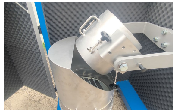
Bond ball mill tilted for unloading
