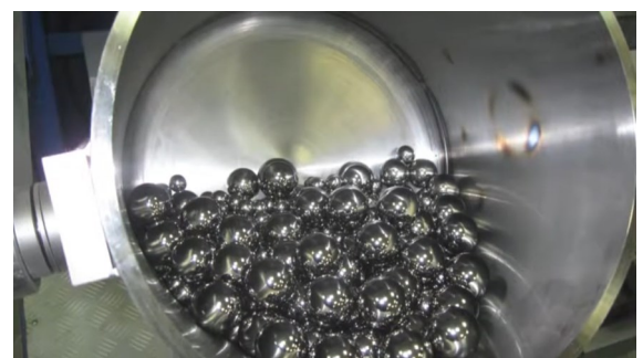
Bond ball mill drum with grinding balls
